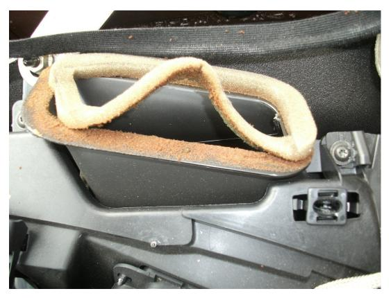
An easy fix, purchase a roll of sticky backed automotive foam 12mm x 6mm. The closed cell type is superior. Simply clean off the powdery residue on the outlet and stick on the new foam.
