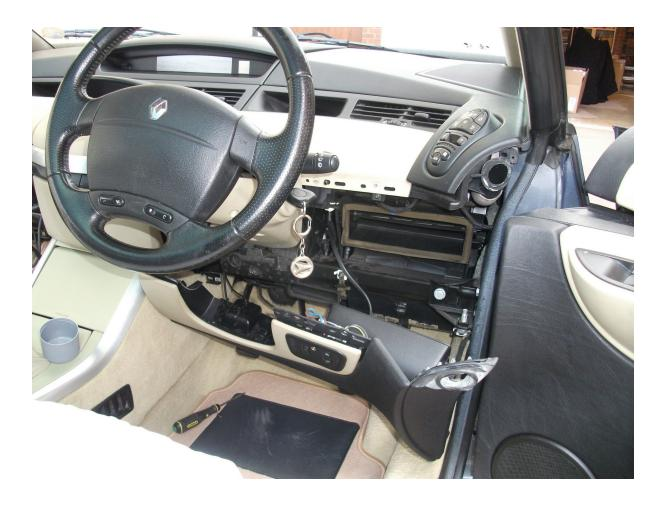
Then feel under the dash for a small 8mm screw head that secures the climate control panel and using a socket or nut runner remove from both sides.
