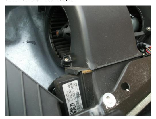
However, to get at it, the nearside fan housing has to be disassembled (4 posidrive screws) and removed. The resistor pack can be jiggled out without removing the fan but it is probably easier to remove it. Disconnect, unclip (large metal clip over the top) and remove. The unit can then be slid forwards and out of its housing (just enough slack on wiring) and then the wiring unclipped.
