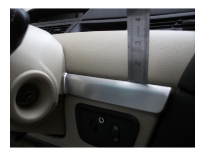
This is probably the hardest part, as the metal trims are very delicate. The most difficult one the passenger side with the 'SRP Airbag' badge. You cannot prise the trim off at this point, it is fixed by a torx screw behind the badge. **But** you cannot remove the badge because you need to access the clips behind the trim! The answer is to slide something thin and flexible but stiff up under the RIGHT outside edge of the badge and feel for the clip. I used a 10thou feeler gauge.
