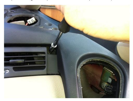
Next prise off the gold coloured spire fastener in the middle of the tacho/vent assembly (photo), pull the assembly upward to free it from the clips, then reach under the lower edge and disconnect the plastic ball and socket holding a plastic actuator rod to the airflow control wheel.
