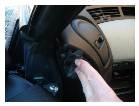
Drop the panels away. If you want them out of the car, remove the wiring to the switches, footwell lights and sat nav CD unit,
