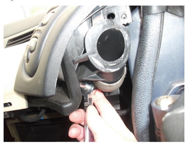
The nearside one is easier to access if you first remove the bracing bar bolted to the body. It is held in place by one 13mm bolt.
