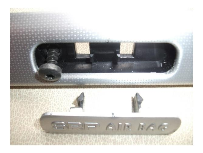
Sometimes the metal spring clips holding the trims fall in to the dash area as you pull the trims out. Don't worry, you can retrieve them from the lower panels once they have been removed.
