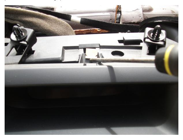
Once the assembly is free you can access the two screws holding the tachometer display to the panel as seen below. It's a good chance to clean the perspex display screen properly using water with a very small trace of washing up liquid. The same applies to the main dash display.
