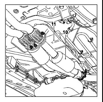
Detach the cables from a clip inside the exhaust tunnel, if necessary.
