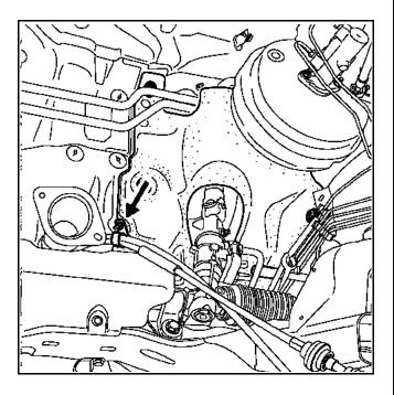
Remove the cable plate and clearly mark the position of the cables.
