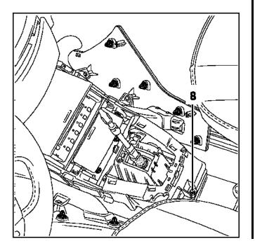
Unscrew the hexagonal nut (8) and the two upper mounting bolts (9).
