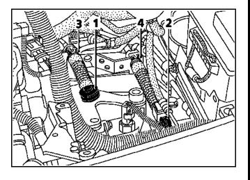
Pinch the sleeve stop retaining clips (3) and (4) and pull upwards to remove them.
