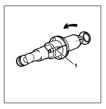
Operating from the passenger compartment, turn the master cylinder clockwise until it locks with the union pointing upwards.
