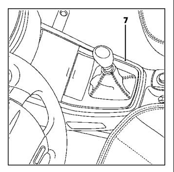
Unclip the gear shift lever gaiter and remove the two rear console mounting bolts.
