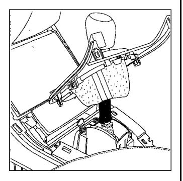
Detach the sides from the central console front section and disconnect the ventilation ducts.
