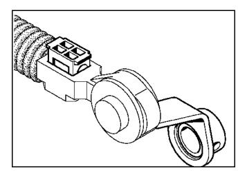
Place the gear lever setting jig (13) on the control lever, using the lever trim housing as support.
