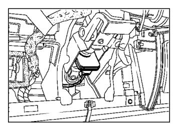
The steering wheel angle sensor cannot be separated from the steering column. You cannot replace the sensor without also replacing the column.
