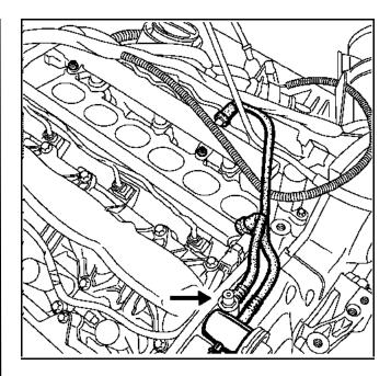
The fuel pressure is regulated according to the atmospheric pressure, not the manifold pressure.
