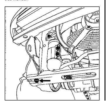
Detach the exhaust pipe underneath the Y-shape union of the catalytic converters.
