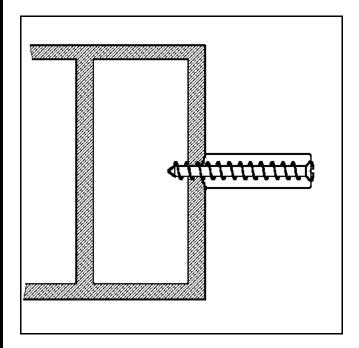
A "Parker" bolt goes through the pin in the shaft and screws into the foot of the radiator, at the base of the pin, which has been pierced to the diameter of the bolt centre prior to the operation. This operation can only be performed on a radiator whose pin has been cut without damaging the foot, and only if the remaining thickness is sufficient for the bolt to "hold" in the metal (approximately 1 bolt centre).
