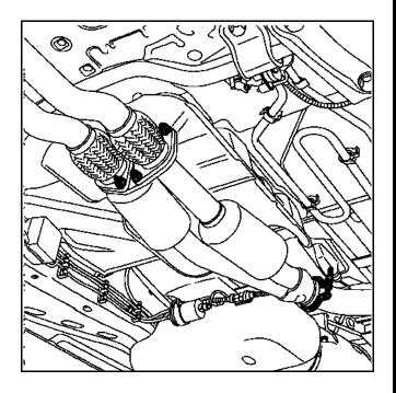
You must remove the torque reaction arm before removing this component, so as to let the exhaust system give way slightly.
