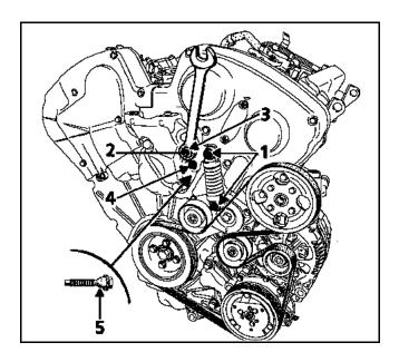
To refit, move the tensioner back into its operating position to the right, and torque tighten bolts (4) and (2) to 2.5 daNm.
