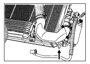
Check that the radiator is not pierced, warped or dented and possibly leaking before starting the operation.
