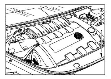
Remove the eight mounting bolts from the upper section (1) and unscrew the clamp (2) on the flexible hose to reach the filter element.
