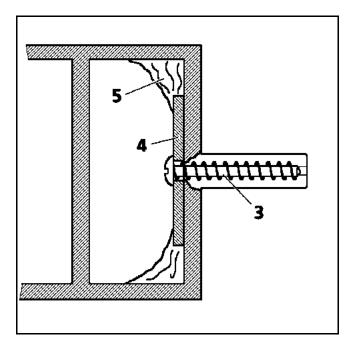
A "Parker" bolt (3) is assembled with the largest available flat washer (4) before being inserted into the surface removed from the foot. The original pin is then screwed into the bolt thread. Use a hacksaw blade, or similar tool, to support the bolt head. Add adhesive (5) to strengthen the assembly.
