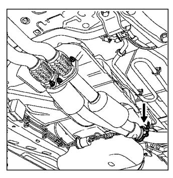
Carefully tip the engine - gearbox assembly towards the front to reach the sensor and then disconnect the sensor electrically.
