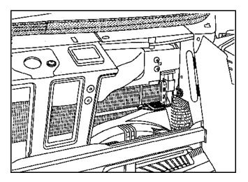
Position a board under the front of the vehicle to support the lower cross member while gaining access to the mounting bolts on the side member tips.
