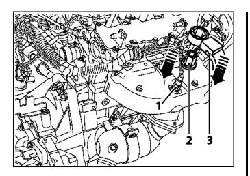
Place the socket (2) around the sensor wiring (1) with the slot pointing downwards (diagram A).
