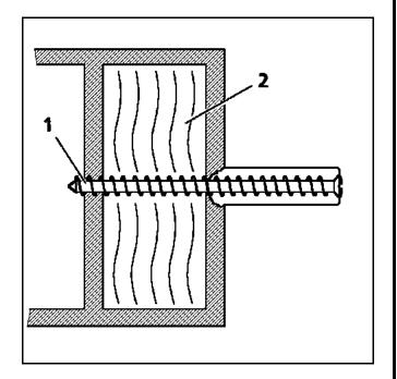
The "Parker" bolt should go through another intact surface on the foot of the radiator (1).
