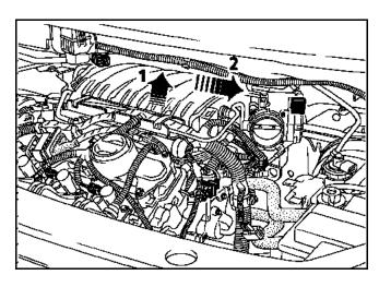
Still pushing to the left, twist the inlet manifold to disengage it between the brake fluid tank and the engine. While twisting, disconnect a temperature sensor behind the inlet manifold.
