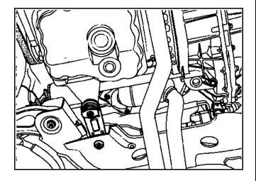
the central catalytic converter assembly rear mountings on the exhaust system,
