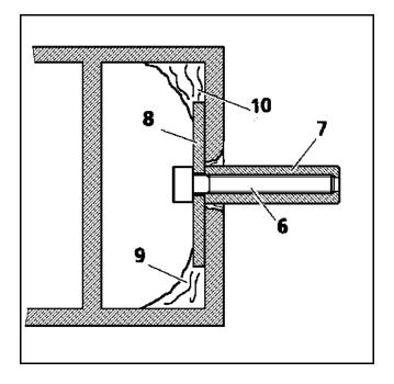
A CHC bolt (6) reinforces a locally manufactured metal pin (7) (with a round rim of the same diameter as the original pin), holding a large flat washer (8). Adhesive (9) strengthens the assembly.
