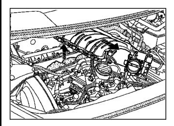
Retrieve the manifold seal from the distributor.
