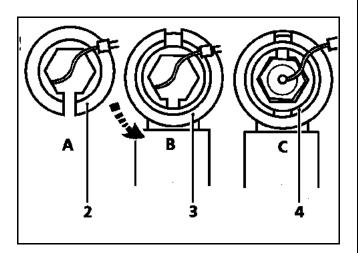
Considerable force is needed to unscrew this assembly, and it is therefore very important to fit the parts in the order described above so as not to damage the tool or the sensor.
