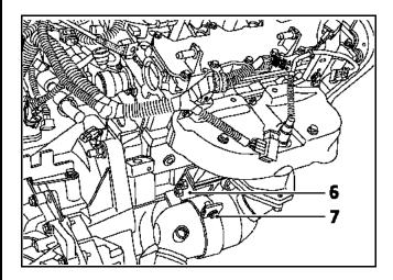
**WARNING**: when refitting, tighten the nut (7) last, after tightening the flange nuts (5) and the bracket (6).
