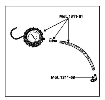
Start the engine. Measure the pressure which should be between  $\mathbf{3.5} \pm \mathbf{0.2}$  bar.
