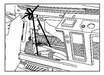
Remove the mounting bolt from the cross piece on the side member.
