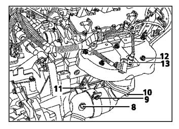
Remove the sensor (13) with tool **Mot. 1610**, from underneath the vehicle (see page 17-3).
