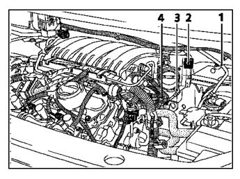
Remove the inlet manifold mounting bolts.
