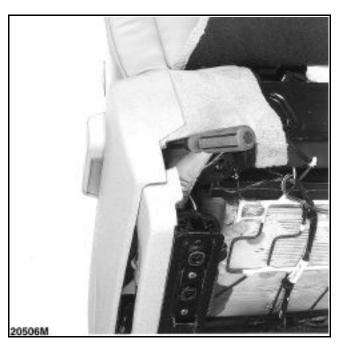
**WARNING:** this handle must be replaced after each operation.
