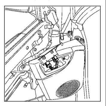
Remove the speaker bolt by turning it a quarter of a turn.
