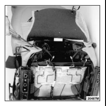
Unclip the retaining profiles and the front lugs.
