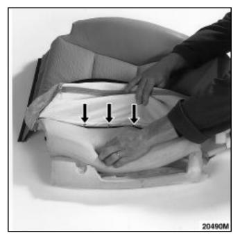
Turn the seatback over and unclip the horizontal seams.
