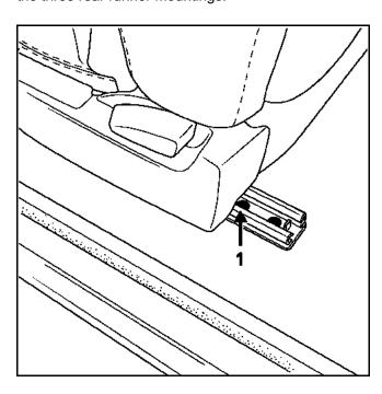
Disconnect the pretensioners and the power supply to the electric seat.
