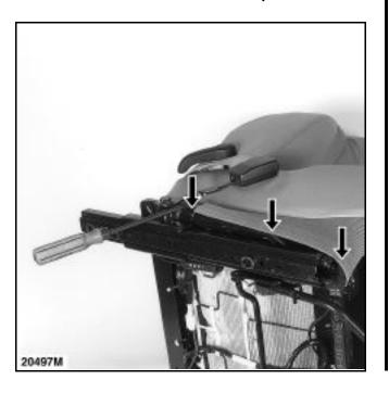
Remove the right retaining profile on the seat belt catch side.
