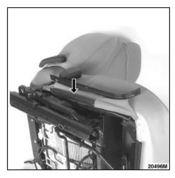
Disconnect the two connectors and cut the plastic clip
