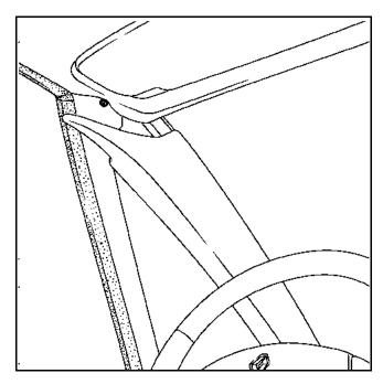
Remove the trim by pushing it upwards underneath the roof trim.
