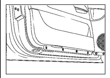
Pull the lining towards you to release the clips, then pull it upwards.
