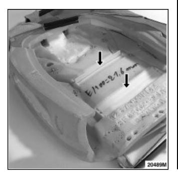
If it is necessary to replace the lumbar heating cover, it is essential to also replace the foam.
