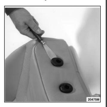
Unclip the retaining brackets on the side air bag and the seatback cover retaining lug.
