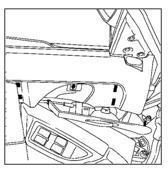
Remove the four lower mounting bolts.
