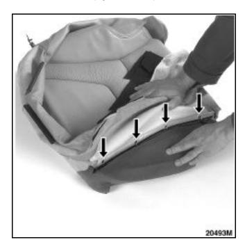
If it is necessary to replace the heating cover, it is essential to also replace the foam.
