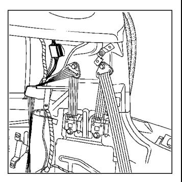
Unclip the cover and disconnect the rear-view mirror and rain sensor connector (if vehicle so equipped).
