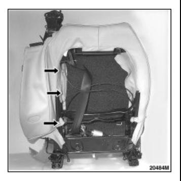
Unclip the cover retaining profiles.
