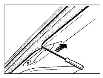
Replace the seals using a thin screwdriver.
