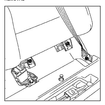
Tilt the seat cushions and remove the four seatback mounting nuts.
