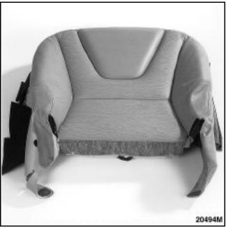
Separate the cover from the foam by removing the cover, then cut the "pig's snout" clips at each seam.
