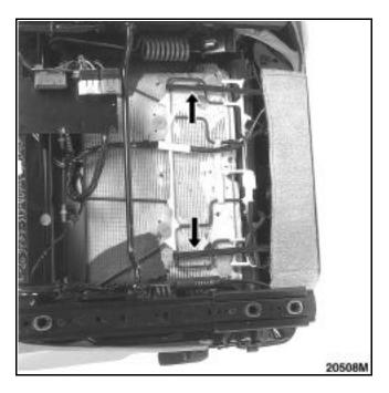
Remove the seatback section by pulling it upwards in order to release the lugs.
