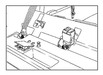
Remove the seat belt catches and the side seat belt anchorages.
