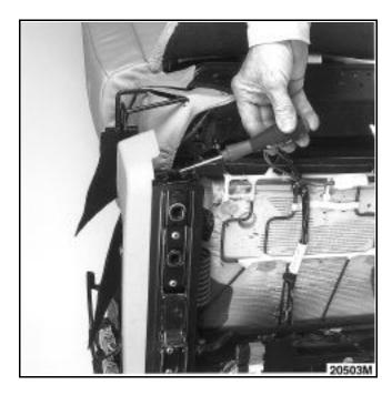
Lift the rear of the housing and pull upwards.
