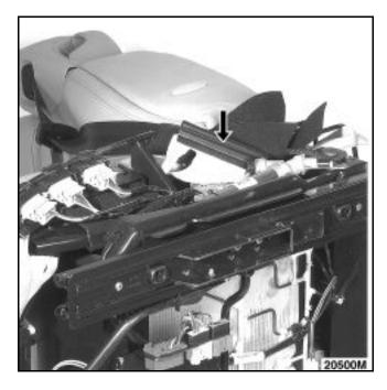
Release the seatback cover retaining straps by cutting the "pig's snout" clips.
