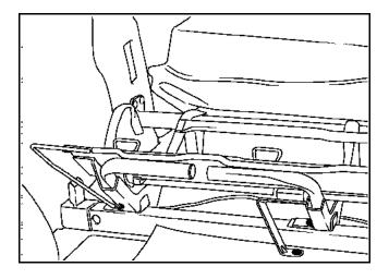
Remove the four rear mounting bolts.
