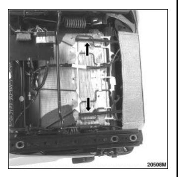
Remove the seat back inclination adjustment handle from the inside by spreading the grooves in the handle with a screwdriver and pulling it upwards.
