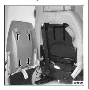
Remove the central trim in seatback tilt handle using a small screwdriver, then remove the handle by pulling it upwards.
