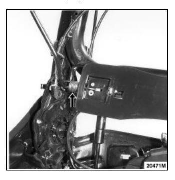
Remove the cable from its housing.
