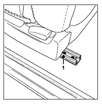
screw the other four seat mounting bolts to the floor finger tight but do not tighten.
