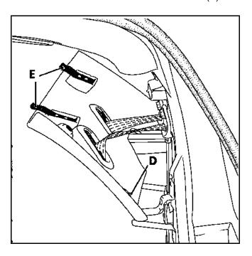
Remove the fixed section of the seat belt.
