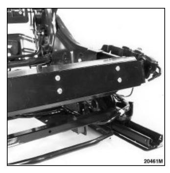
Release the flexible rod by pulling it straight from the connector on the motor end.
