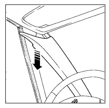
Disconnect the roof harness connector.
