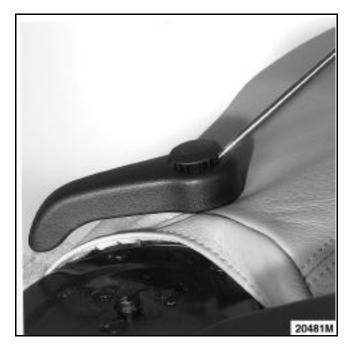
Remove the head rest by lifting the lug.
