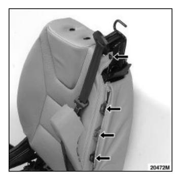
Unclip the seatback cover retaining clips by pulling them towards the outside of the seat.
