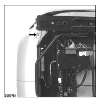
Pull the housing upwards.
