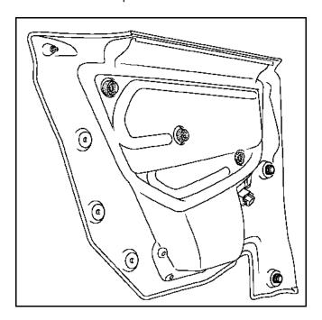
Carefully lift the lining in order to release the upper section of the window seal.
