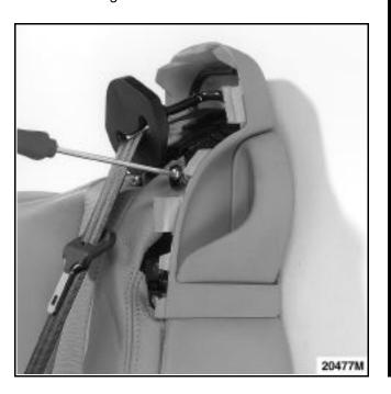
Remove the pin of the seat tilt handle.
