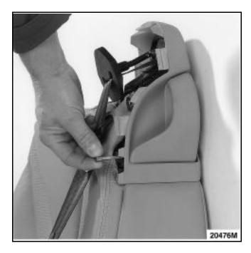
Remove the handle by pulling it in the direction of the arrow.
