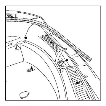
Remove the four mounting bolts for the lashing rings (Torx  ${\bf 30}$ ).
